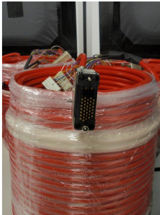
Radial and SAMTEC connectors for one of the 140' HV supply cables
